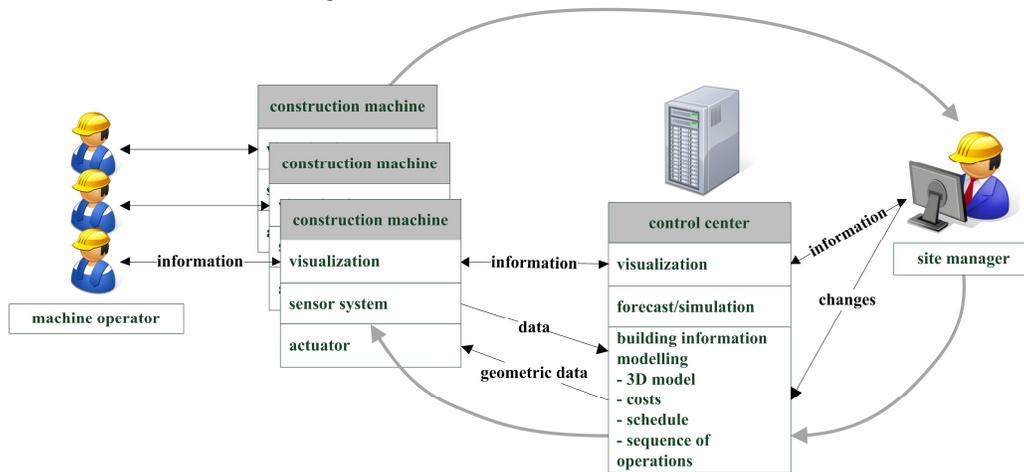
Figure 3: control center architecture
