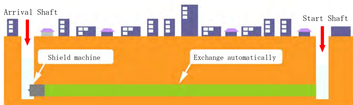
Figure 1 Cutter bit exchange image figure by the double bit
