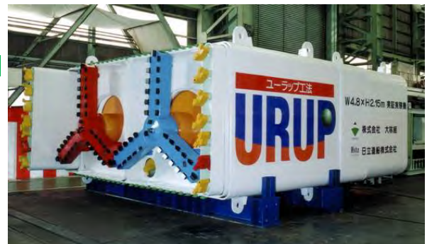
Photo-1 URUP Method Proving Test Shield Machine
