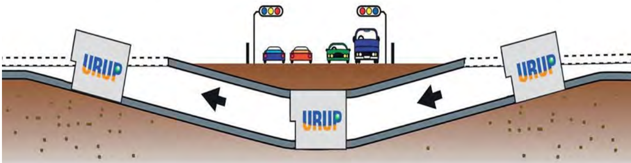
URUP method – Shaftless Shield (Shield Tunnel Boring Machine to launch and arrive at the ground level without vertical shafts)
